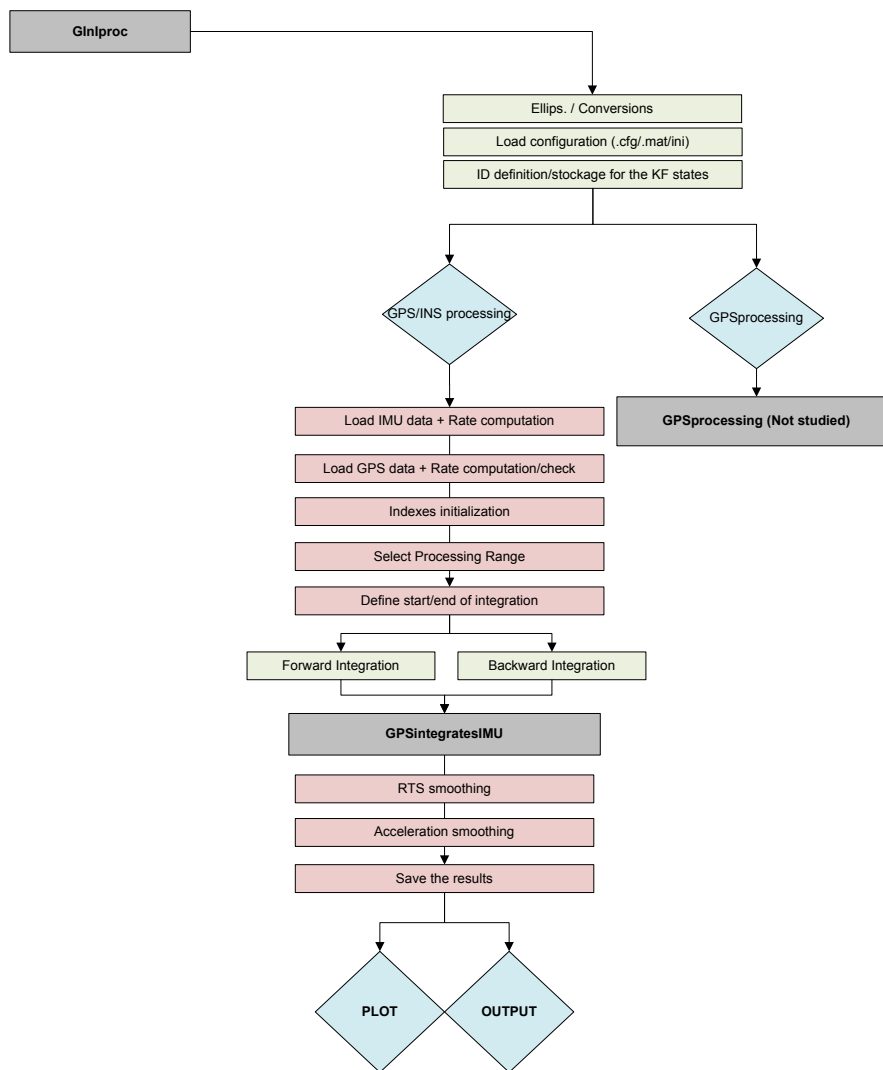
Fig. A.2: Flow chart of the software's main algorithm
