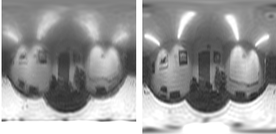
Fig. 15: Reconstructed full spherical images without correction of the registration error (Left) and with the joint registration and super-resolution with Levenberg-Marquardt algorithm (Right).
