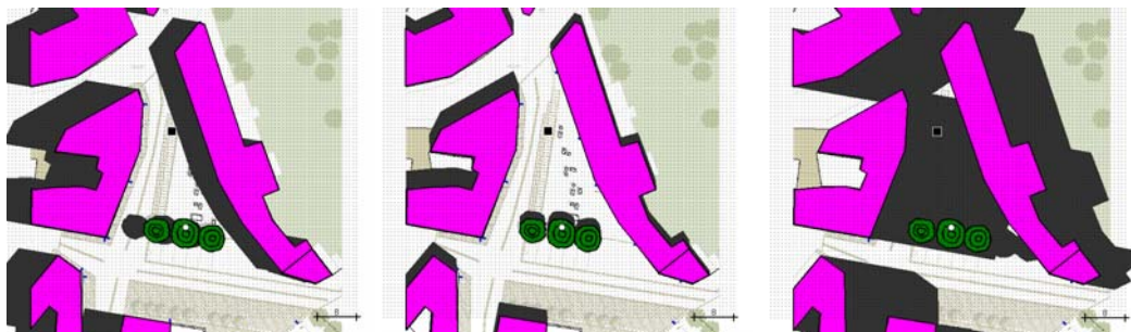
Figure 7: The shadow analysis through the shadow brought by the buildings
