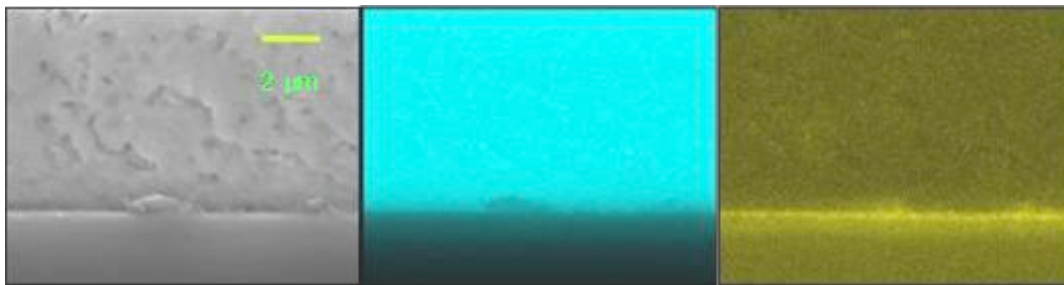
Figure 4: Interface analysis of SnAl10.6% m bonding specimen
