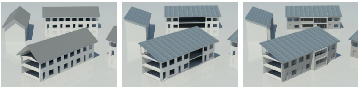
Figure 2: Visualization of the renovation process; the existing structure (left), the stripped structure with the Solar Roof (middle) and the new building envelope (right).
