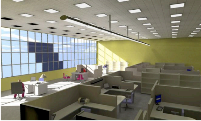
Fig. 3: The WALLDOW outer shell is divided into arbitrary units which will be individually controlled according to the desired needs of each workstation. Occupants will have an option to individually control the shading of their space.
