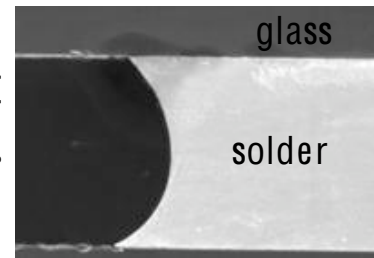
Figure 3c: SEM inspection of the bonded interface
