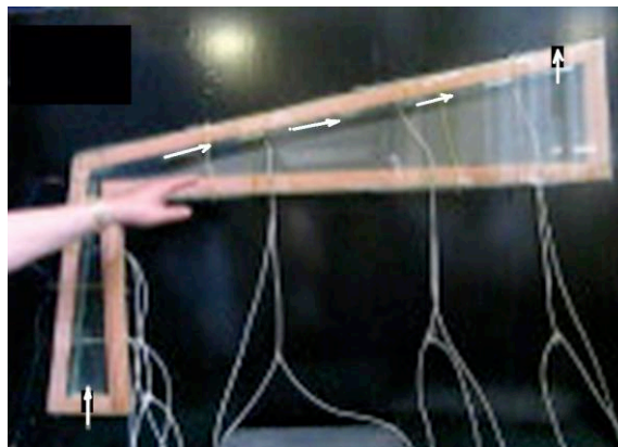
Figure 5: Air flow image with tracer gas (grey smoke)
