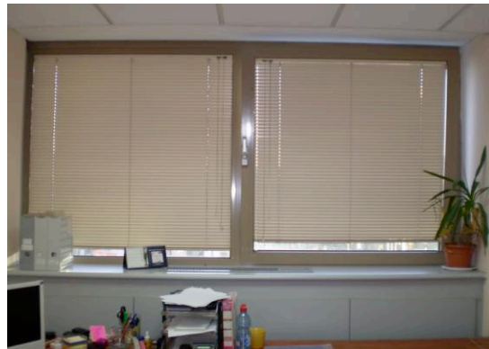
Fig. 2: An interior view of a window in one of the offices of Figure 1. The shades are almost completely closed. Occupant has left a narrow opening to allow some daylight get in and have a limited view out. The Electrical lighting is made of 8 Fluorescent luminaires, switched on all day.
