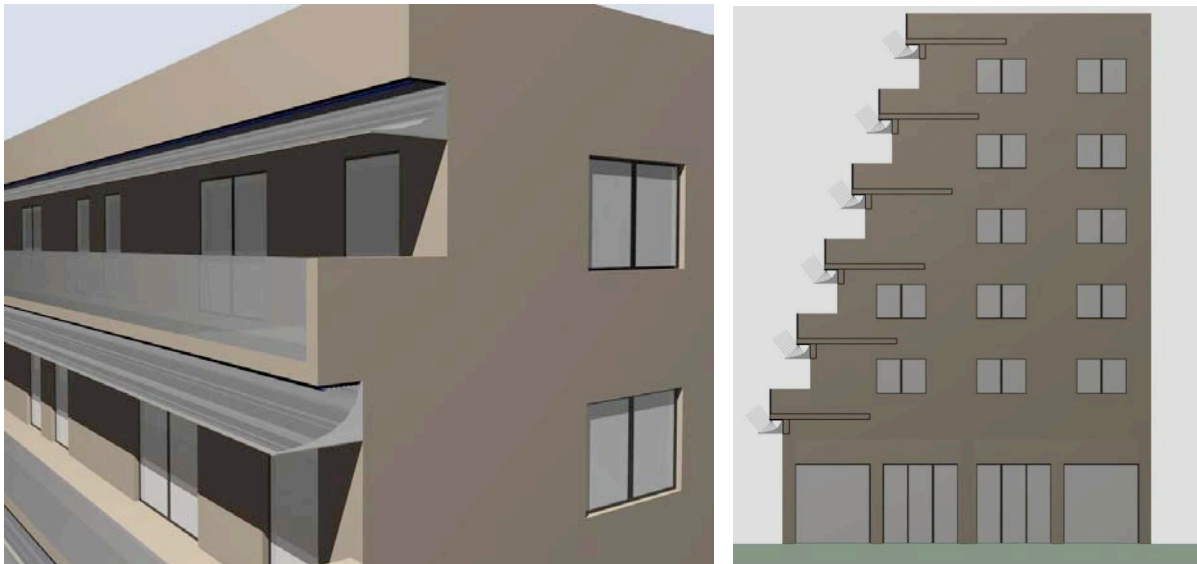
Fig. 9 Building integration of CPC reflectors with tracking PV or PVT absorber on the rear side of the front placed building
