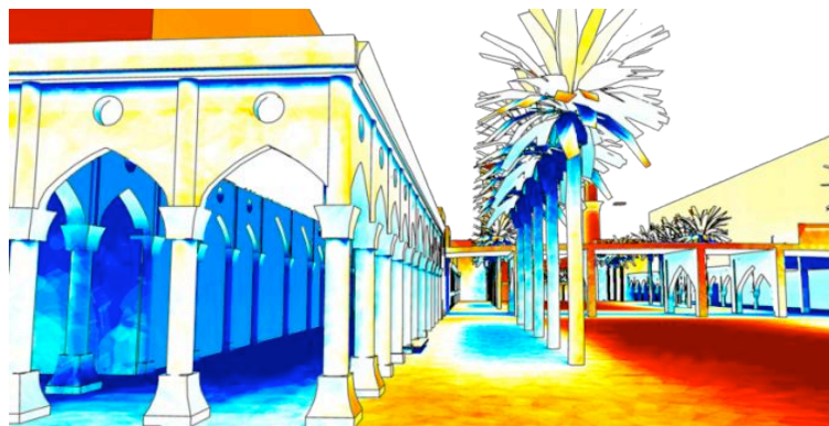
Figure 9: SOLARCHVISION yearly perspective view analysis of Imam Ali holy shrine extension complex which shows the proper effect of porch and trees in this climate.
