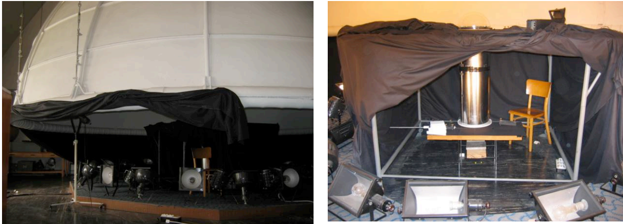
Figure 2: Experimental measurement of light tube transmission under the artificial sky
