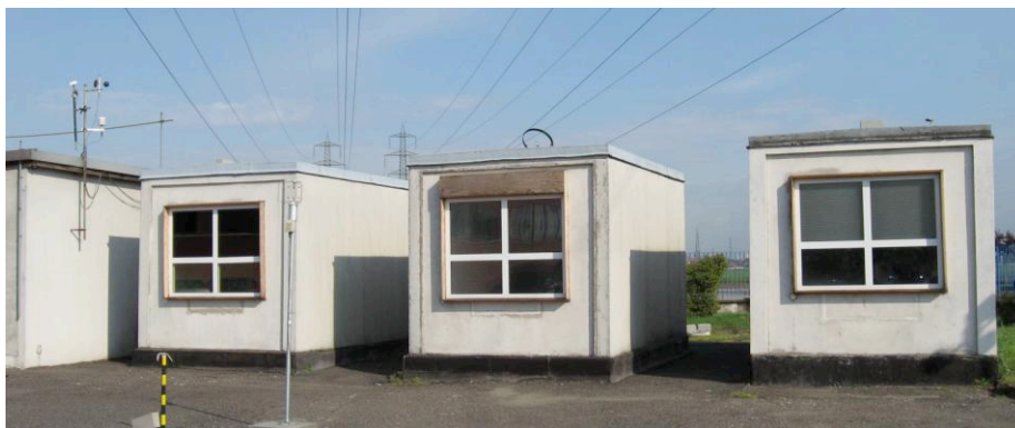
Figure 1: outdoor view of the test cell. The reference room is in the middle
