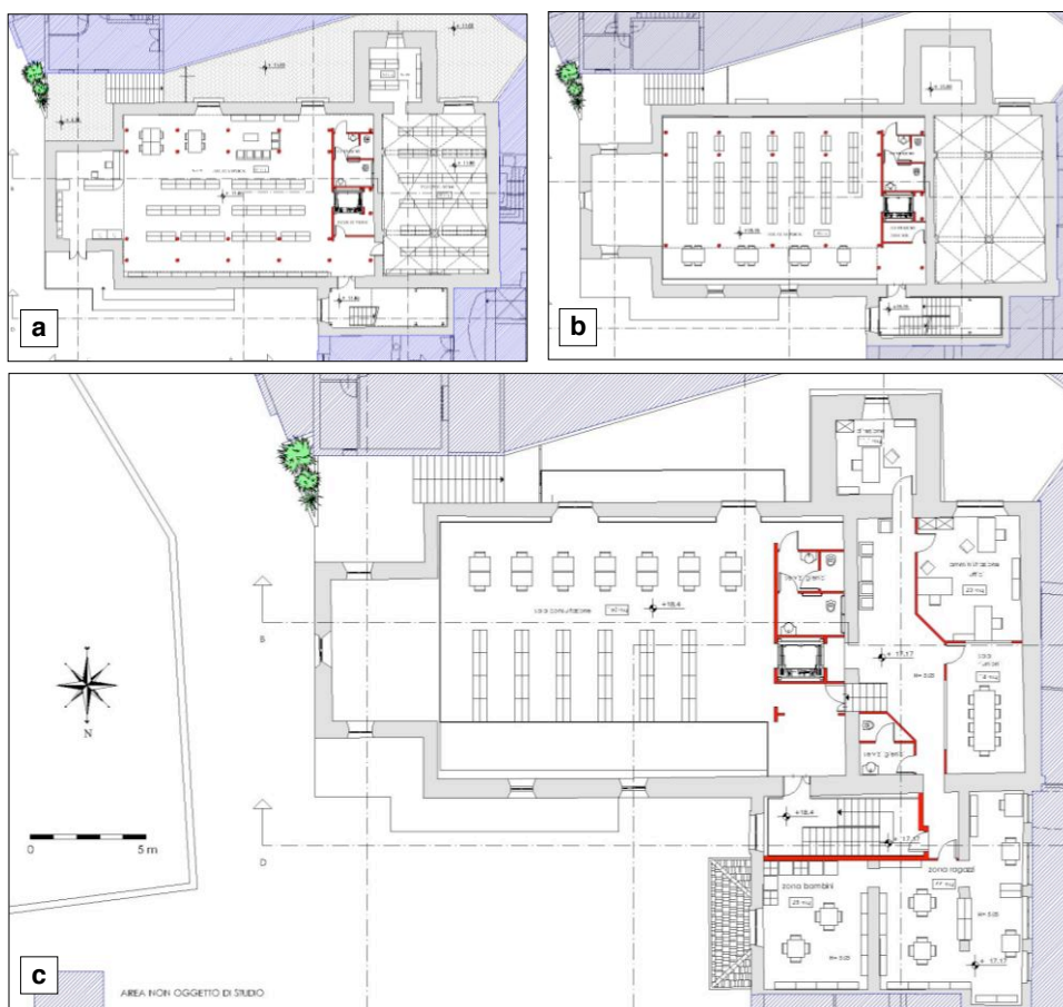
Figure 2– Project drawings [1]: a) Ground floor; b) 1 st floor; c) 2 nd floor (the furnishings positions are shown).
