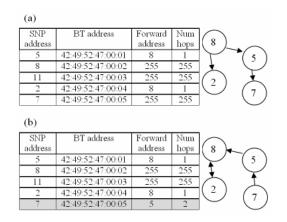
Fig. 4. (a) If a packet should be send to a device to which the path is unknown, the packet as well as a search packet gets broadcasted. (b) The answer packet from the receiver is used to update the friend table.
