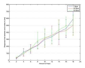
Fig. 8. Delays for transmission of data packets in the wireless Bluetooth scatternet for different numbers of hops in the network.
