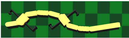
Fig. 8. Posture of the standing wave when higher amplitudes are applied to the limb segments. Notice how this higher bend resembles a possible movement of a pelvic girdle-femur angle (elliptical hip activation).
