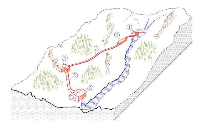
*Figure 2: Main component of a high-head MHP plant (Andaroodi, Schleiss et al., 2005, p. 22)*
