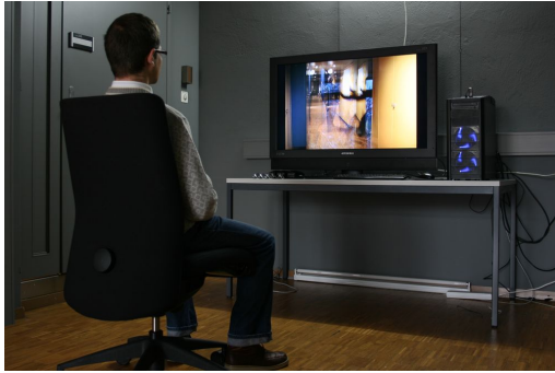
Fig. 4: Quality test laboratory and 46'' polarized 3D display used for the subjective quality evaluation.
