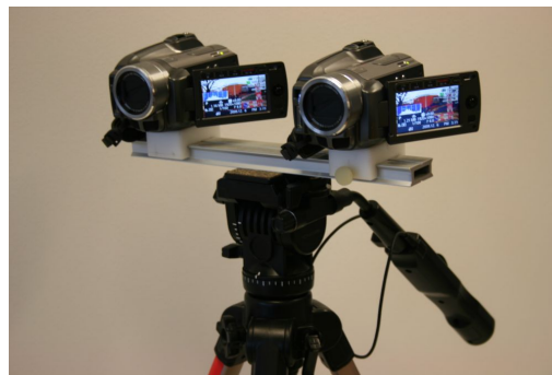
Fig. 2: HD stereo camera setup consisting of two identical camcorders and an adjustable stereo mount.
