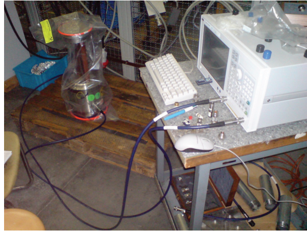
Figure 5.47: S-parameter measurement setup for the BPH.
