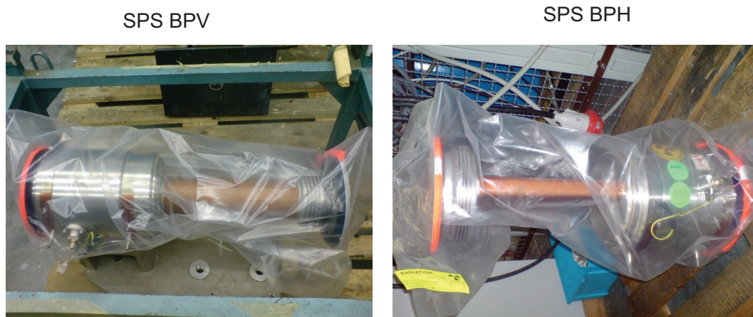
Figure 5.46: SPS BPV (left) and SPS BPH (right) used for the S-parameter measurements. The sealing plastic bag around the BPMs had to be pierced to plug the cable in the N ports connected to the electrodes.
