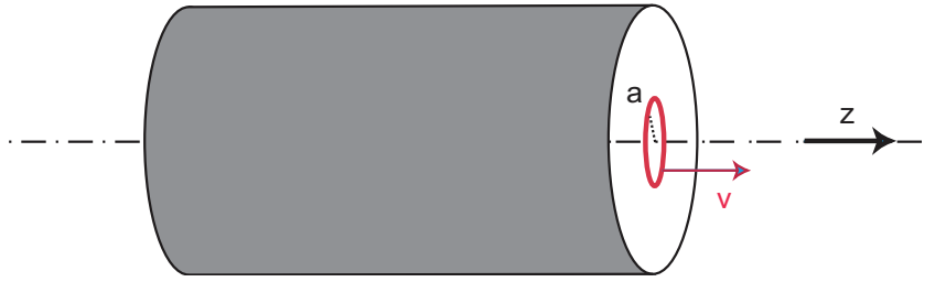
Figure 5.1: Sketch of an annular beam of radius a moving with velocity \vec{v} parallel to the z -axis.
