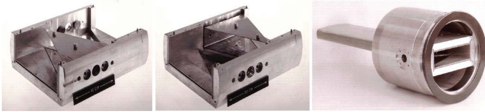
Figure 5.37: Pictures of an SPS BPH: partly dismantled BPH inner body (left and center) and full BPH assembly (right). The triangular-shape electrodes and the white ceramic spacers on top of the electrodes are visible on the pictures of the dismantled inner body.
