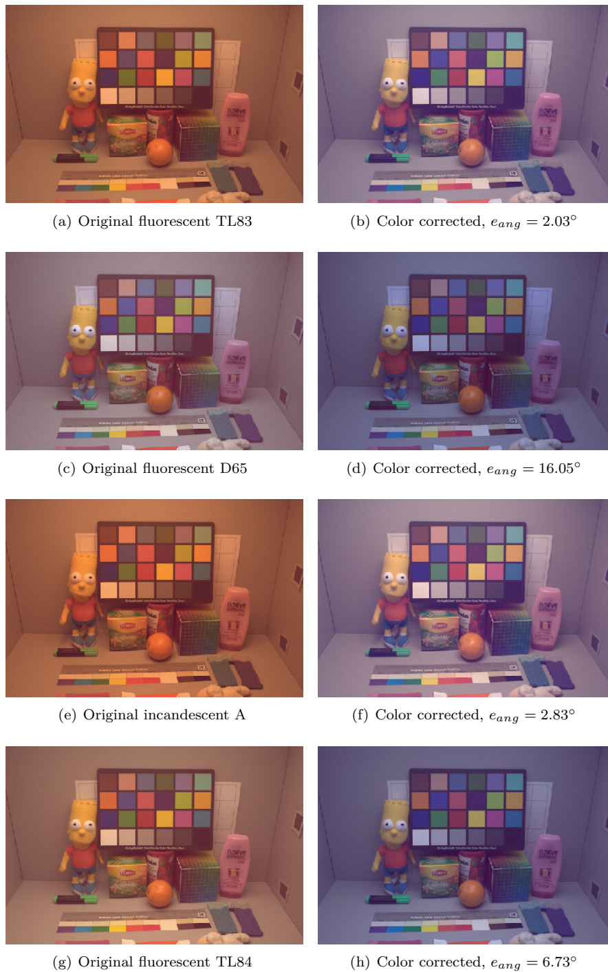
Figure 5.21: Lightbooth images used in Examples 1 and 2. The images in the right column are corrected using the retrieved illuminants displayed in Figure 5.20.
