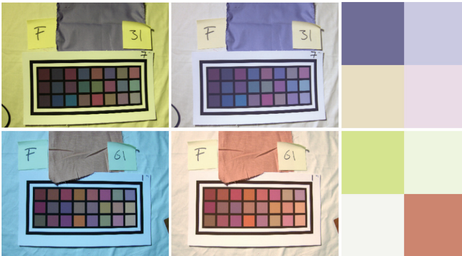
Figure 4.3: Paint samples are grouped in palettes of four colors. The system matches the object color to one of the paints and returns the corresponding palette. The figure shows, from left to right, the uncorrected image, the corrected image, and the corresponding paint palette.
