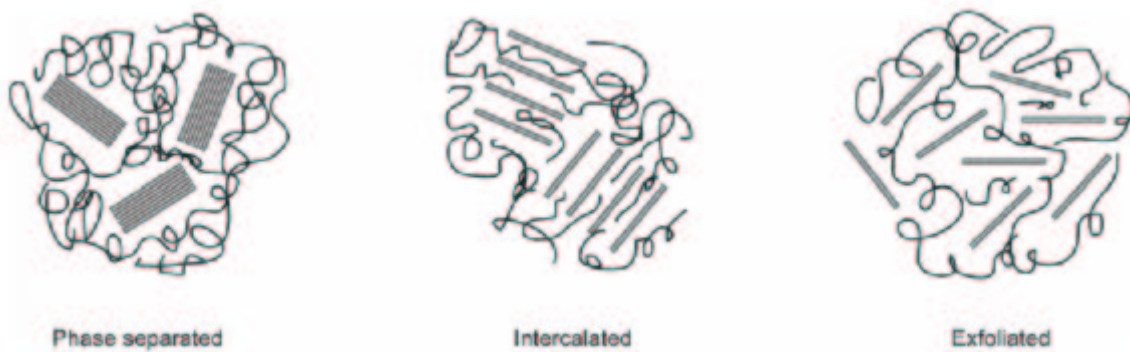
Fig. 2.2 Typical morphologies of layered silicate clays in polymer matrices [1].
