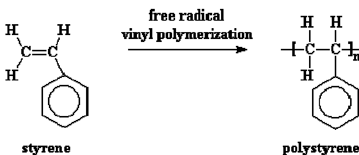
Fig. 3.3 Schematic of the polymerization reaction.
