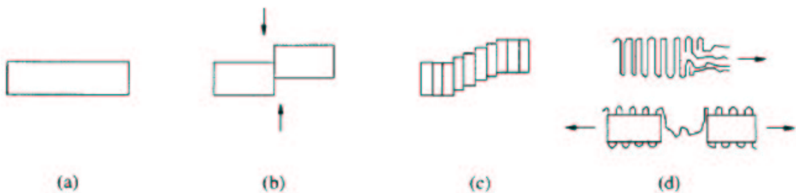
Fig.2.19 Deformation of polymer crystals: (a) undeformed state, (b) block slip, (c) fine slip, (d) chain unfolding and lamellar break-up.
