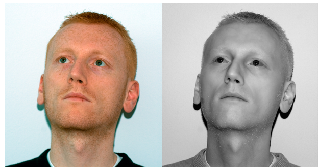
Figure 1. Visible and NIR representation of a portrait. While the skin appears much smoother in the NIR, all the high-frequency details are effectively preserved.
