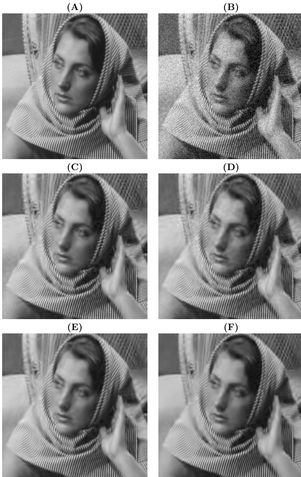
Figure 4.10: (A) Part of the noise-free Barbara . (B) Noisy version of it: SSIM = 0.48. (C) Denoised by UWT-ProbShrink : SSIM = 0.85. (D) Denoised by DTCWT-BiShrink : SSIM = 0.86. (E) Denoised by FSP-BLS-GSM : SSIM = 0.87. (F) Denoised by the proposed pointwise SURE-LET , optimized in an UWT/BDCT dictionary: SSIM = 0.88.
