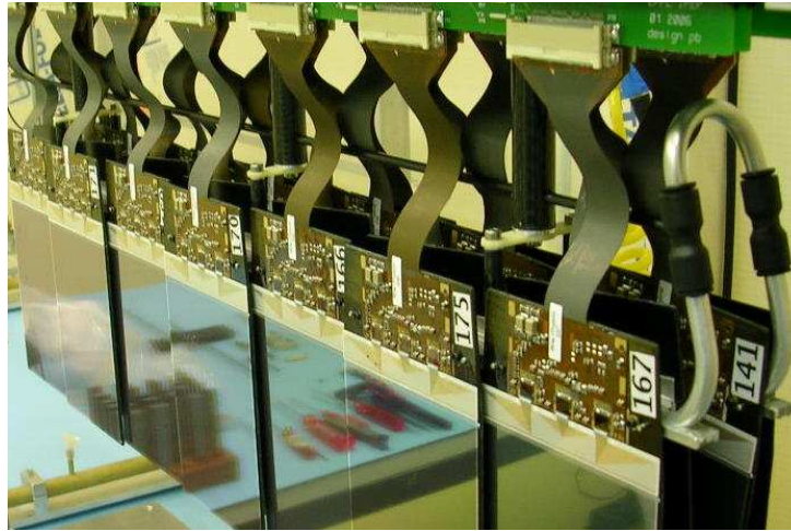
Figure 5.18: Photo of the IT layers fixed to the aluminium cooling rod. Both the X and stereo layers are visible, as well as the cooling-rod bending on the right of the picture.
