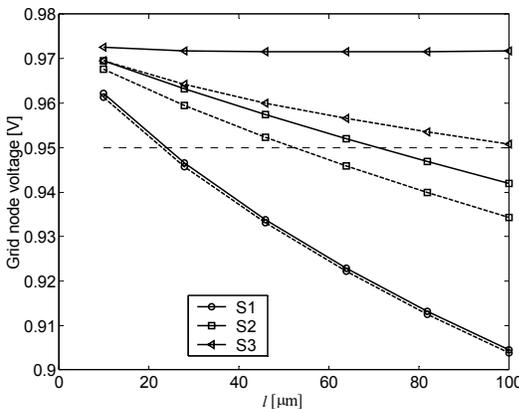
**Figure 11.** SPICE simulations of the voltage drop on M1 grid for different nodes and with no stack of vias removed ( $d = 0$ ) with (solid curves) and without (dashed curves) the TSV path. Only three current sources switch.
