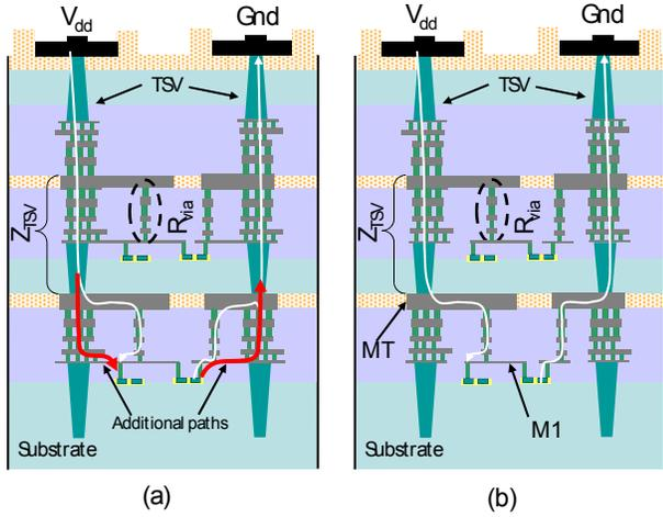
**Figure 3. Current paths within a 3-D circuit, (a) where the TSV is connected to the power lines on both the uppermost (MT) and the first (M1) metal layers and (b) where the TSV is connected only to the topmost (MT) metal layer.**
