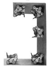
Figure 5: The robot moving from floor to ceiling
