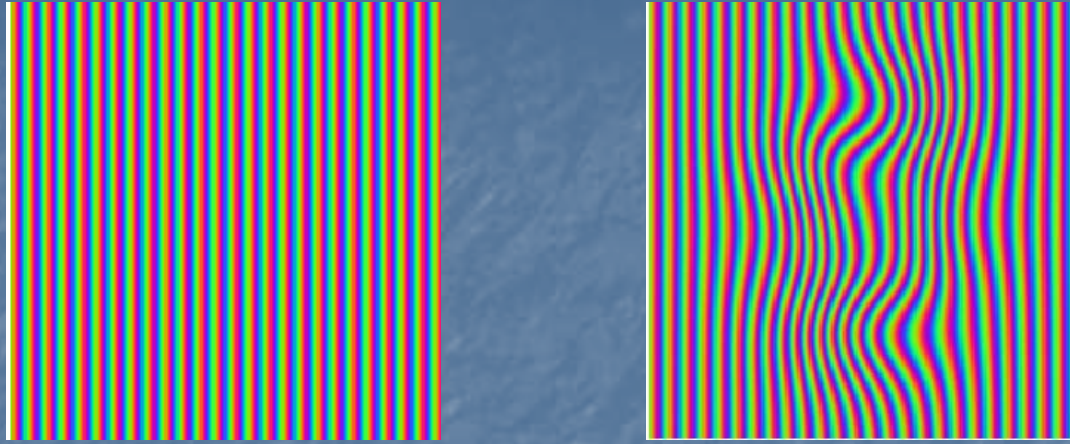
Figure (a) RGB color encoded fringe pattern on reference plane (b) the deformed fringe pattern when projected on to the object surface.
