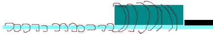
Figure 10: Here a schema of the sample mounting is shown. The resistor (black) sits behind the \text{LiHo}_{0.04}\text{Y}_{0.96}\text{F}_4 -crystal. The Cu-wire insures a good thermal conductance. The whole system is then put into styrocast.
