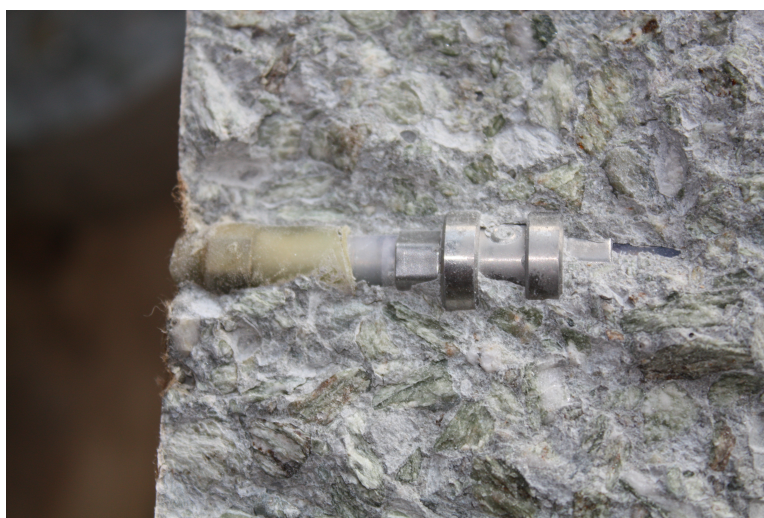
(b) Photograph of the sensor after the sample has been split in a Brazilian test.
