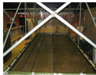
Fig. 1. The EPFL erosion flume divided into 4 smaller flumes
