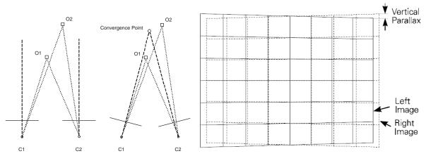
Figure 5. Parallel(left) and toed-in camera configurations(middle) with a typical keystone distortion due to toed-in camera configuration(courtesy of <sup>21</sup>)
