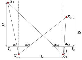
Figure 2. Formation of image points and effect of depth to disparity
