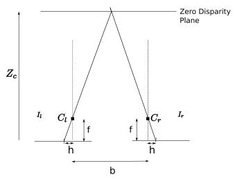
Figure 3. Image Plane shift for disparity adjustment and zero plane setting.
