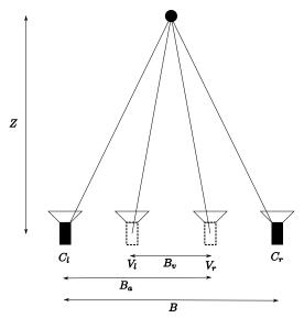
Figure 4. Virtual Camera Configuration for disparity scaling. Actual baseline distance is B. When both left and right images come from virtual cameras, the baseline distance is  $B_v$ . The configuration where only one of the images comes from the virtual camera is called asymmetric synthesis and the baseline distance is  $B_a$
