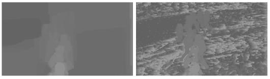
Figure 7. Estimated disparity maps by graph-cut and cost aggregation methods. Note the noisy disparity map by cost-aggregation.
