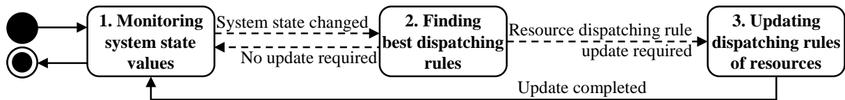
Figure V.10. State transition diagrams of the dispatching rule allocator agent.
