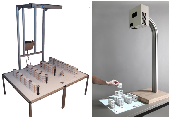
Figure 2: Left: The TinkerTable, a tabletop learning environment for apprentices in logistics. Right: The TinkerLamp, a smaller and lighter version of the TinkerTable.
