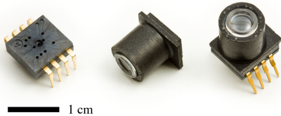
Figure 7: From left to right: the Avago ADNS5050 optic mouse sensor, the custom-designed optics based on the Philips CAX100 collimator lens ( f = 10 mm) and the assembled optic flow detector (weighing 0.8 g).
