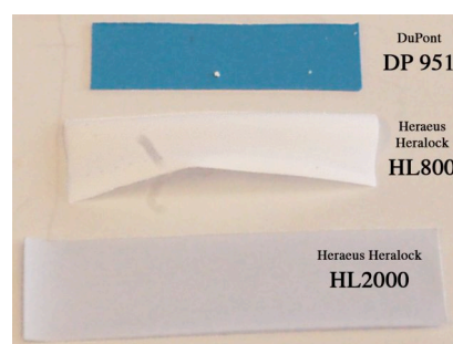
Figure 1. Single fired layers of the three LTCC compositions
