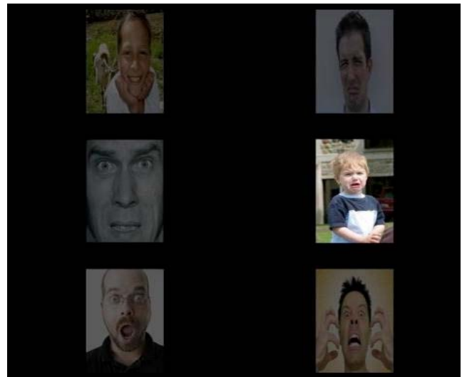
Figure 5. The graphical user interface used to evoke the P300. Images were intensified, one at a time, by modification of their overall brightness.
