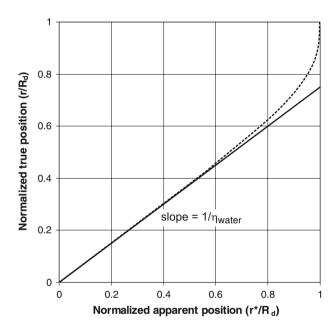
**Fig. 12** *Solid line*: true position versus apparent position of a point inside a water sphere, observed perpendicularly to the straight line connecting it to the spheres center. *Dashed line* linear expansion about  $r = r^* = 0$
