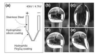
Fig. 7 a Schematics of the electrodes with their coating; b quasi-spherical drop, c oblong attracted drop, d slightly repulsed drop, e strongly repulsed drop
