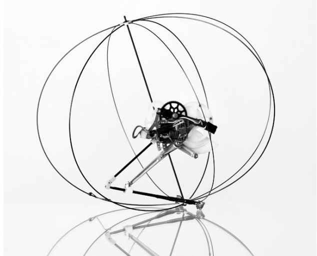
Fig. 1. 9.8g jumping robot able to jump, roll passively, upright itself after landing and jump again. The cage has a diameter of 12cm.
