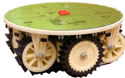
Fig. 2: The base module of the marXbot robot.
