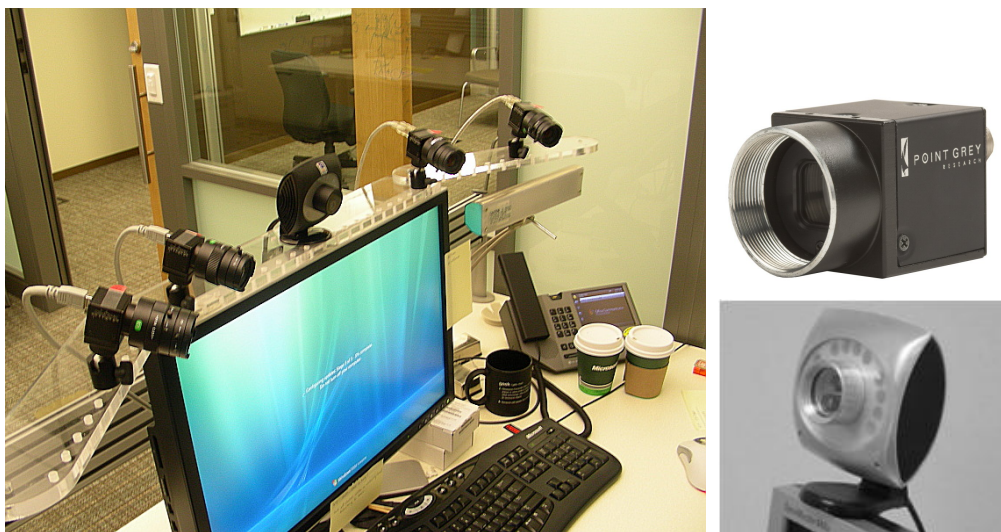
Figure 1: Left: Our hybrid camera system is placed on top of a 22" monitor with 15 degree bent linear extensions. At the center we have the depth camera and the intensity cameras are spread on the grid to cover a large area of interest for a teleconferencing application. Right: On the top, one of the PGR Flea cameras used to capture intensity and on the bottom the infrared based depth camera.
