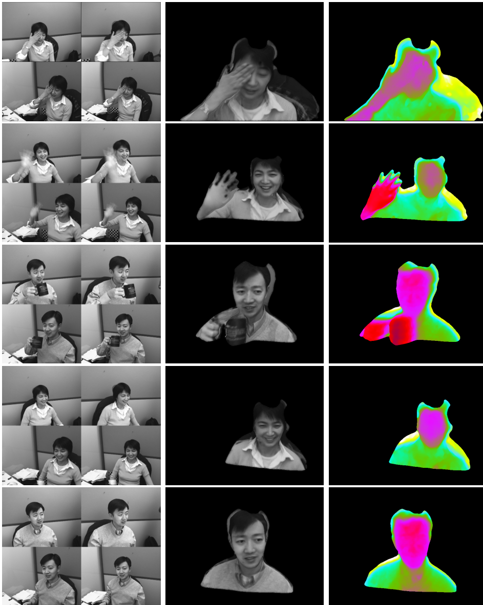
Figure 12: Some Renderings. Here we show the results of our algorithm for some example frames. Within the rows, first 2 \times 2 image shows the input of the cameras, middle column is our result and last column is the computed depth map. We see that even for some challenging cases, like the first 3 rows, our algorithm produces decent results.
