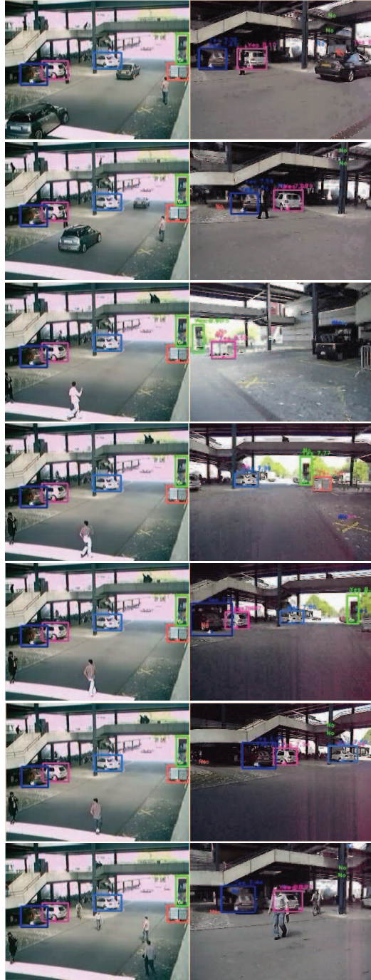
Figure 26: Correct detections and no false positives. First column: objects detected by a fixed camera. Second column: corresponding objects detected and matched with a mobile camera
