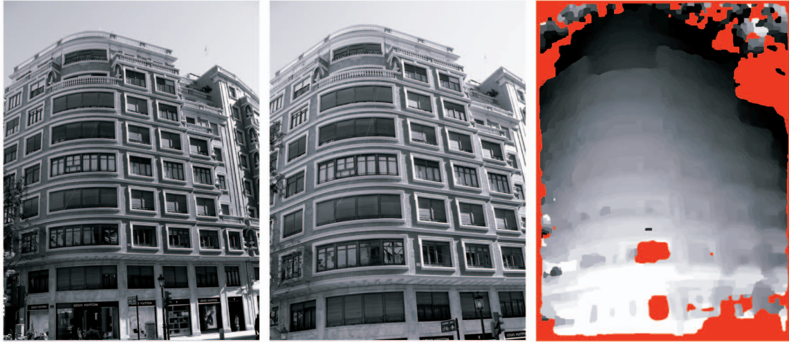
Fig. 19. Brightness Change: We compute the depth map from the second image's point of view using DAISY. There is a brightness change between the two images.
