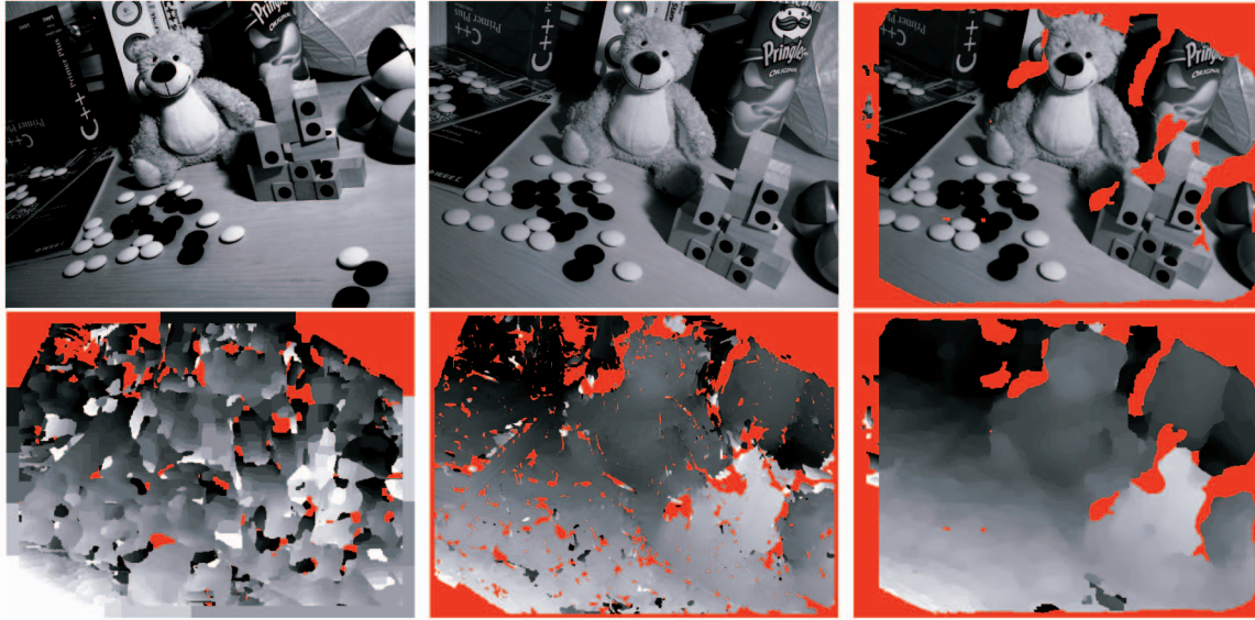
Fig. 1. Contrast Change: The first two images are used as input. We manually increased the contrast of the first image and tried to estimate the depth from the second image's point of view. We used NCC, SIFT, and DAISY, and their reconstructions are displayed in the second row, respectively. We also resynthesized the second image using the depth map of DAISY and the first image's intensities and show it at the end of the first row.
