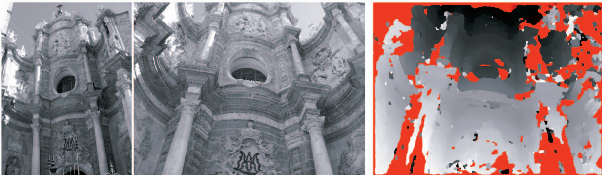
Fig. 18. Valencia Cathedral: The reconstruction results of the exterior of the Valencia Cathedral from two very different viewpoints. The depth map is computed from the second image's point of view.
