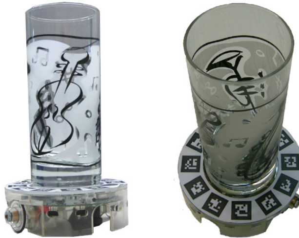
Fig. 1 Interactive and mobile drinking glasses merging the role of glasses and mobile robotic technology. Lateral and top views.
