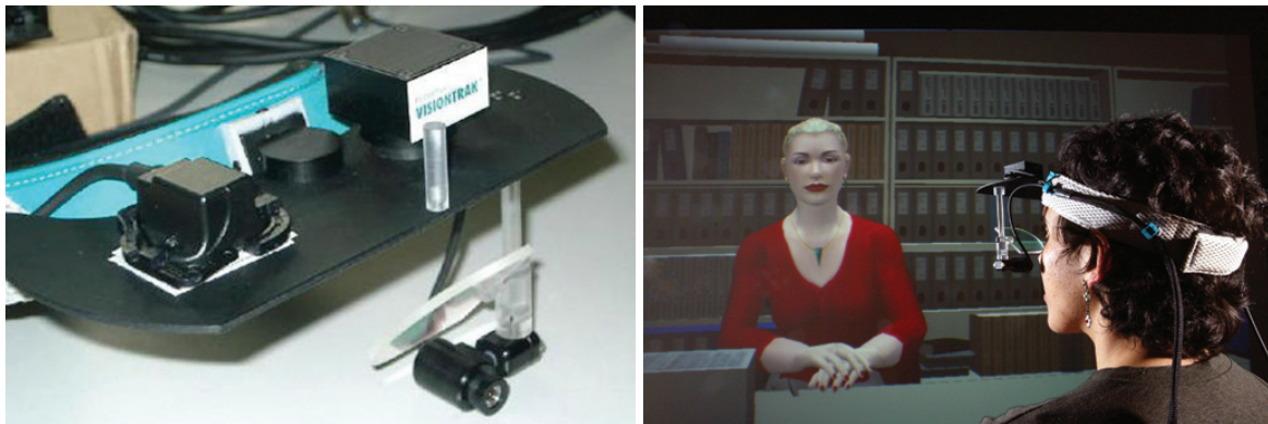
Figure 6.2: Eye-tracking device, Left: eye-tracker. Right: subject wearing the device, seated in front of the back-projection screen ( Photo: Alain Herzog ).
