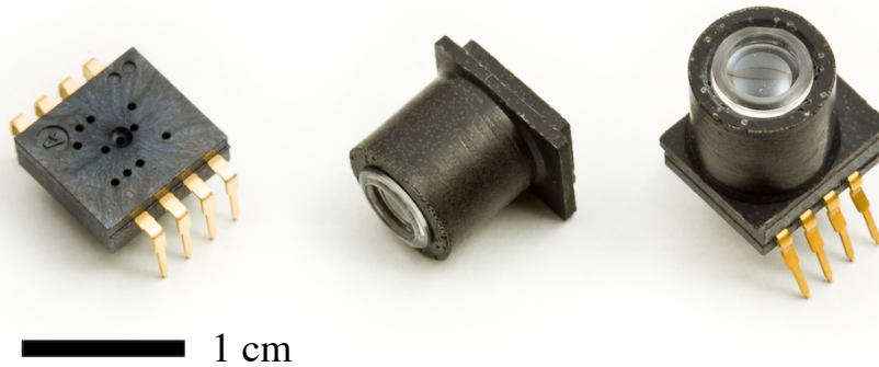
Figure A.4: From left to right: the Avago ADNS5050 optic mouse sensor, the custom-designed optics based on the Philips CAX100 collimator lens ( f = 10 mm) and the assembled optic flow detector (weighing 0.8 g).
