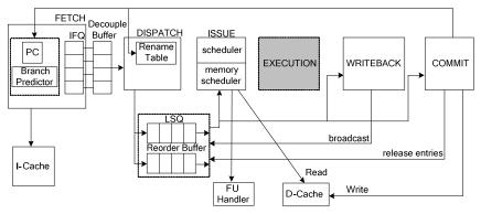
Figure 1 ReSim Block Diagram.
