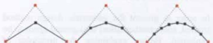
Figure 5. Iterative construction of a Bezier curve
