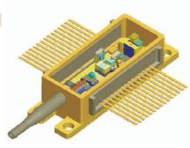
Figure 1.1: Optical transceiver currently built at Intel (Courtesy Intel Corporation).
