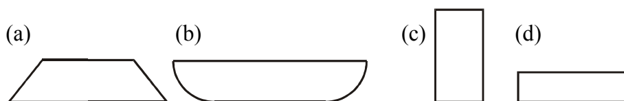
Figure 1: Several types etching profile are obtained by varying the etching conditions. (a) KOH-wet etching of silicon, (b) HF-wet etching in \text{SiO}_2 substrates and (c, d) DRIE.
