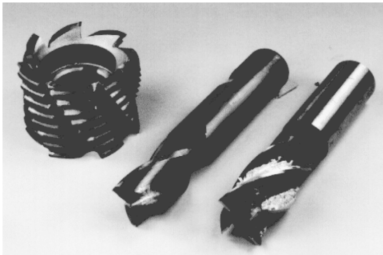
DLC coated drills (source: IWS-FHG)
