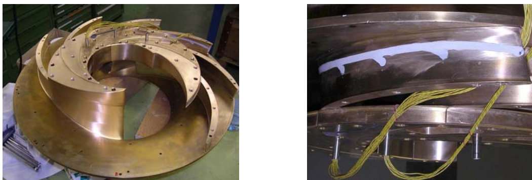
Figure 3.3: Assembly of the instrumented impeller
