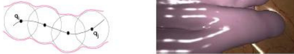
Figure 8: Modeling intestine with spheres for fast collision detection (France, et al. 2005).
