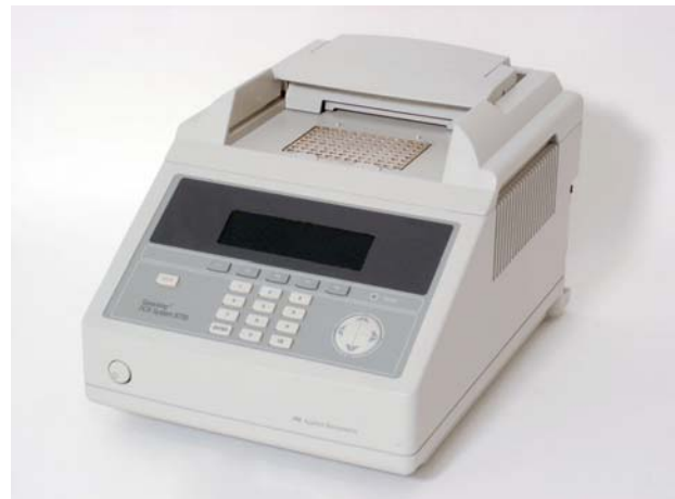
Fig 47. One thermal cycler (Applied Biosystems, USA) used for PCR amplification in this manuscript.
