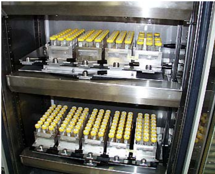
Fig 14. TubeSpin consisted of 50-ml ventilated centrifuge tubes for small-scale experiments in suspension culture. These 50ml sterile tubes have five openings and one gas-porous filter on the cap to regulate gas transfer. They are small bioreactors, used for large-scale parallel tests, optimization experiments and small-scale suspension culture.
