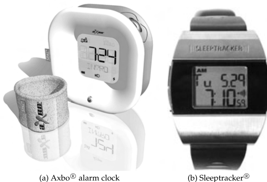
Figure 2.8: 'Gentle wake-up' devices to increase alertness after wake-up based on accelerometer recordings. From Axbo (2008) and Sleeptracker (2007).
