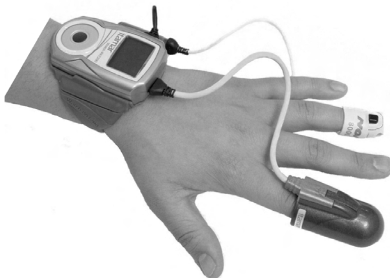
Figure 2.3: The WatchPAT™-200 measures blood oxygen saturation, peripheral arterial tone and activity to discriminate sleep stages and respiratory sleep disorders. It is designed to be used in ambulatory sleep monitoring to detect obstructive sleep apnea, the most frequent sleep disorder. From Itamar (2009).
