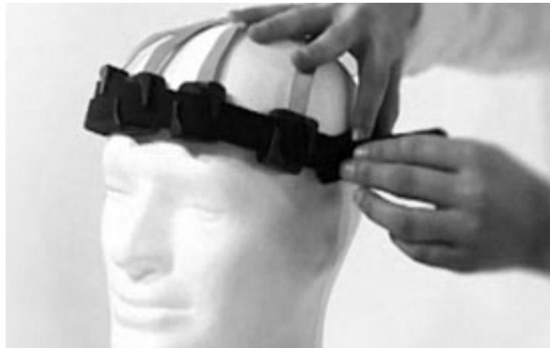
Figure 2.10: ENOBIO ® gel-less sensor system for EEG measurement and on-line sleepiness prediction developed during the European project SENSATION. From Starlab (2009).
