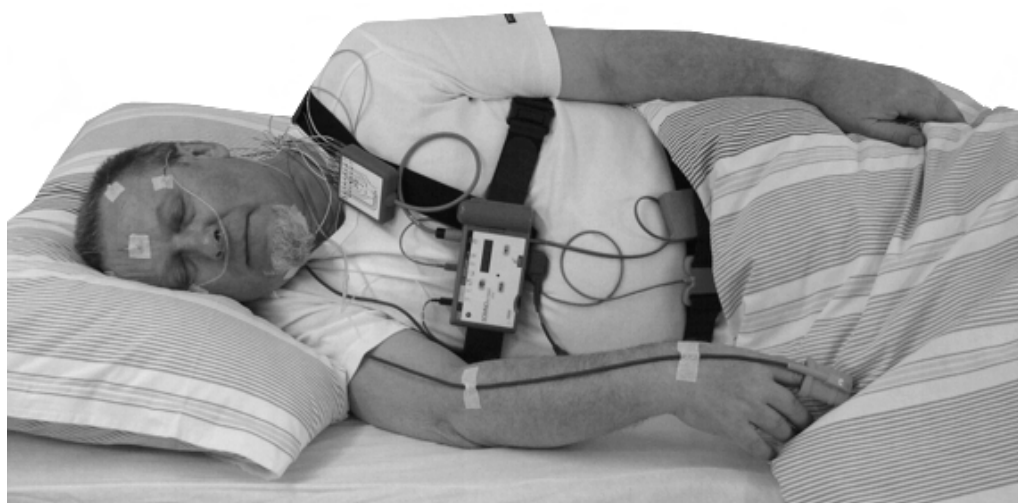
Figure A.1: Portable physiological recording system used for ambulatory sleep screening. The sensors have to be applied by a technician and the cables and sensors need to be glued to the skin. Picture from Somnomedics (2008).
