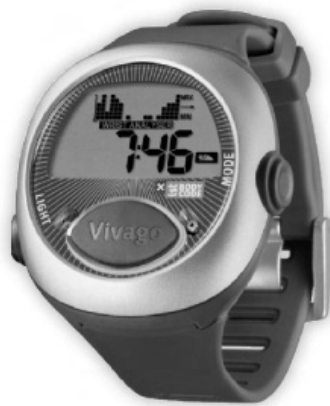
Figure 2.4: Vivago ® Active. An actigraphy based wellness watch that displays past activity, sleep histograms and statistics on the screen. Image from Vivago (2009).
