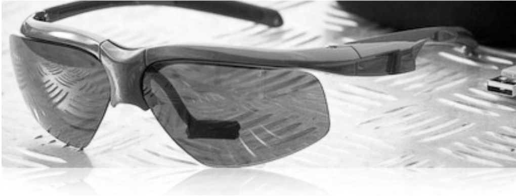
Figure 2.7: Optalert™ alertness detection glasses. IR proximity sensors are measuring the velocity of the eyelid movements to estimate the alertness of the wearer. From Optalert (2009).
