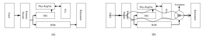
Fig. 1. The (a) SS1 baseline superscalar and (b) SS2 redundant execution microarchitectures.
