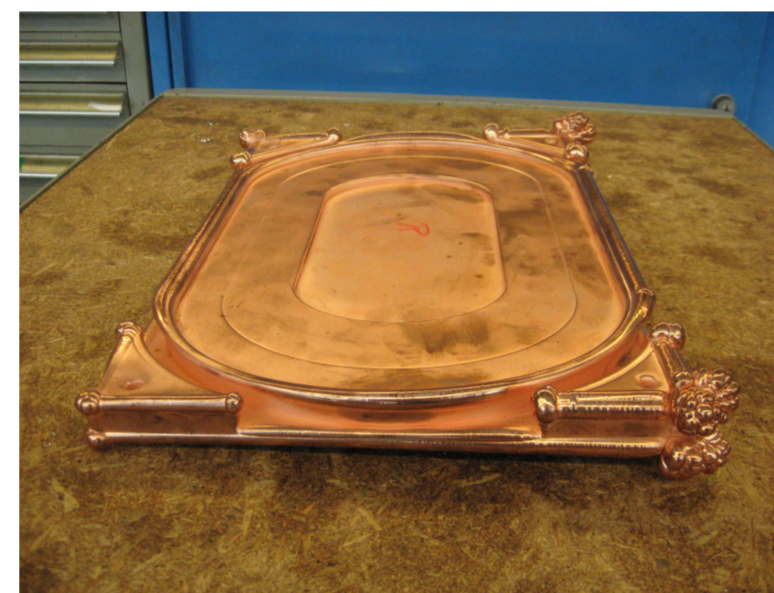
The current density profile makes the deposition rather in the edges than in the center, which is the opposite of the desired Cu profile
