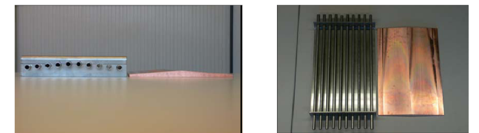
The pre-HIPped prototype mirror assembly consisting of the SS box, cooling tubes and copper mirror as viewed from the a) side and b) top
