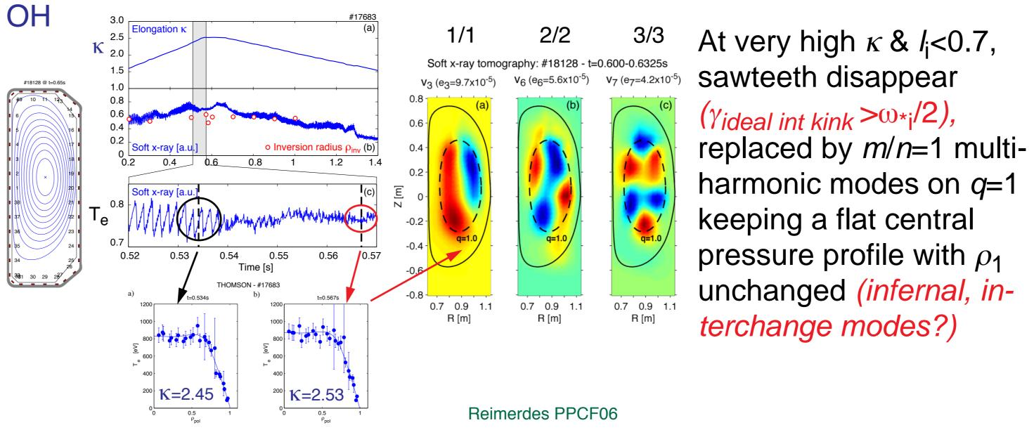
• the limiting pressure inside q=1 ( $\beta_{Bussac}$ ) is determined by shape •  $\tau_{ST}$  follows ideal internal kink stability • parallel to Mercier ideal stability over this shape range
