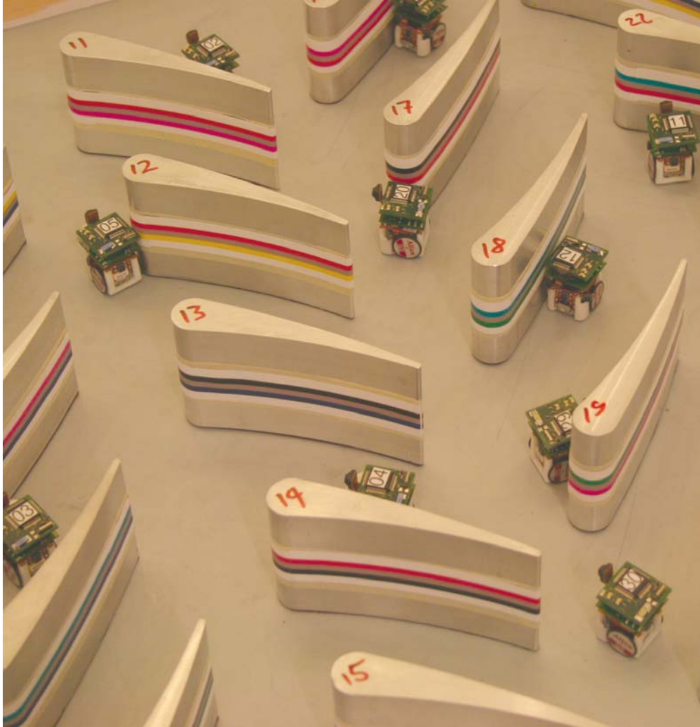
Fig. 3. The experimental setup endowed with colored markers that allow for unique identification of a blade using the on-board camera.
