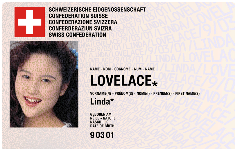
Fig. 12 ID card with geometrically transformed text running over the whole document
