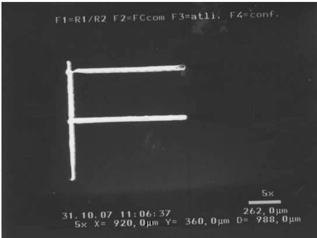
Figure 5. Micrograph of the laser ablation-fabricated microcantilever. It must be noted that the ablation lines (in white colour) are quite accurate, with no thickness change. This suggests that the laser beam energy is efficiently and properly conveyed to the ablation lines. The length and width of the U shape between the ablation lines are 920 \mu\text{m} and 360 \mu\text{m} , respectively.
