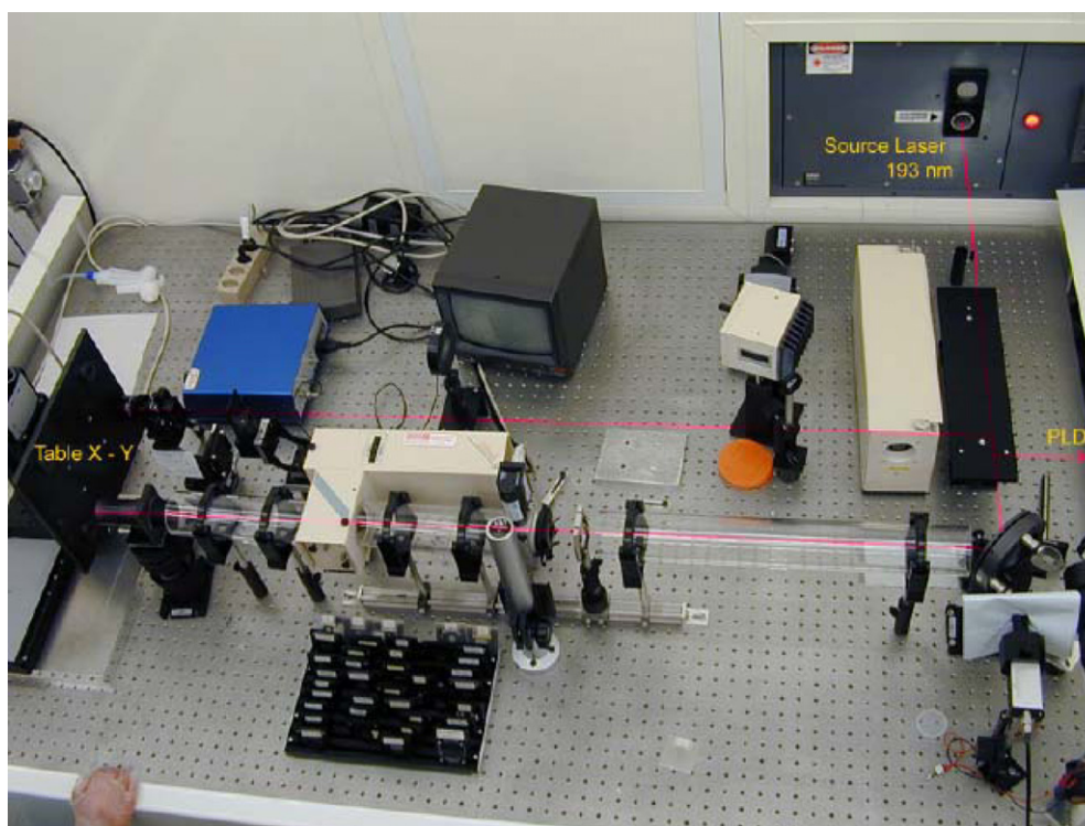
Figure 3. A photographic view of the excimer laser ablation system used.
