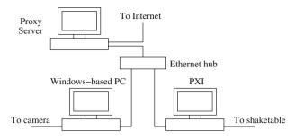
Fig. 2 Network setup of the computers
