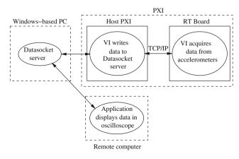
Fig. 6 LabVIEW components for data acquisition
