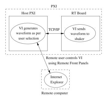
Fig. 4 Wirgau et al.'s [6] framework for shaketable control
