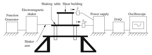
Fig. 1 Laboratory setup of shaketable experiment
