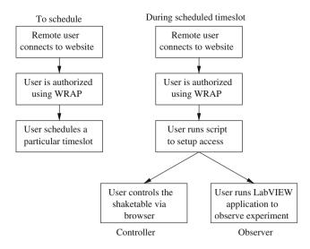
Fig. 8 Flowchart showing remote user actions to access the experiment
