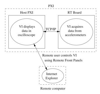
Fig. 5 Wirgau et al.'s [6] framework for data acquisition
